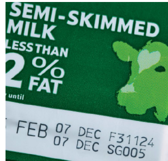
Expiration code Color change on laser sensitive coating of dairy carton film sleeve
